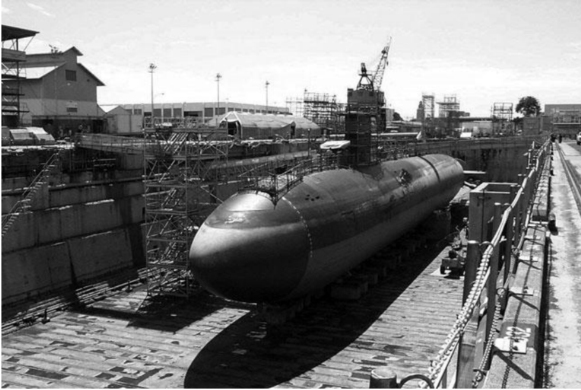
Figure 10.2 USS Greenville sits atop blocks in dry dock at Pearl Harbor naval shipyard following a collision at sea with the Japanese fishing vessel Ehime . (DoD photo.)
